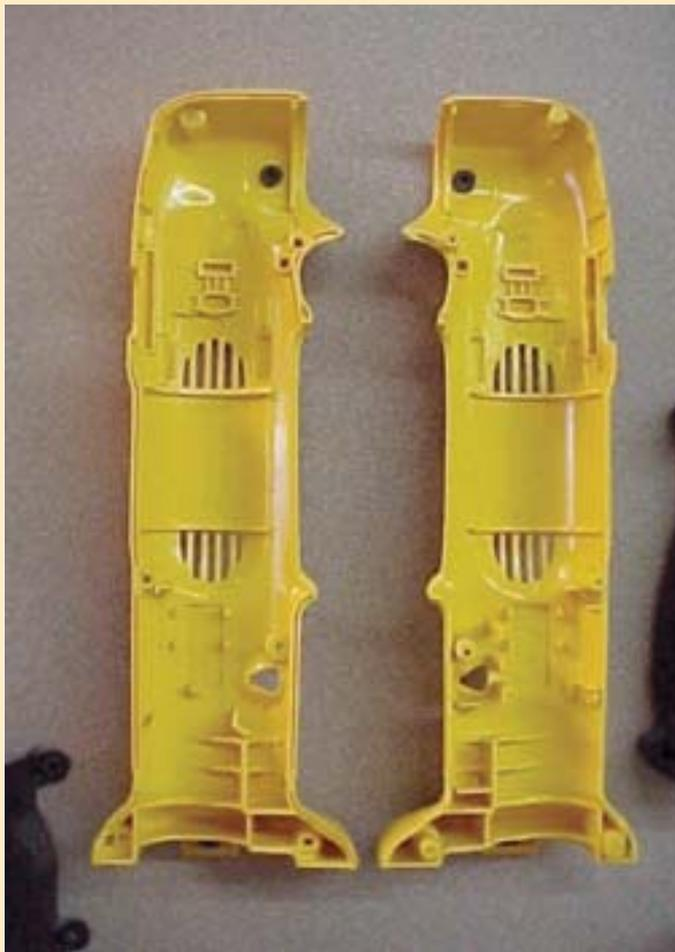
Prototype hand tool clam shell design.
