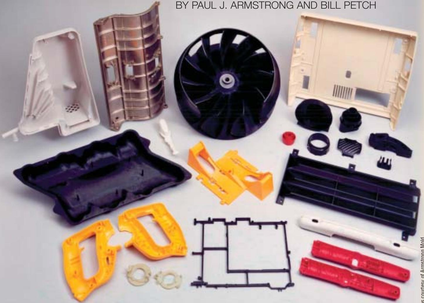
Diverse array of parts run in cast kirksite molds.
